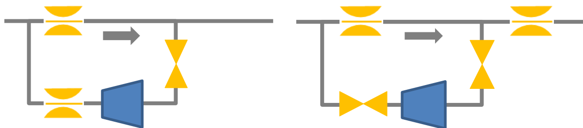
Fig.12 Schematic diagrams of throttling regulation of a hydraulic energy recovery unit
